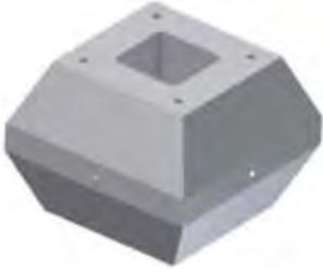
The ArmorFlex® OS system is a variable size, articulating mat consisting of machine compressed concrete units. Each unit is kiln dried, resulting in compressive strengths over 3,000 psi. After the units have been manufactured, mats are assembled by lacing
