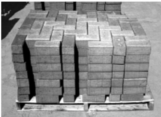
Figure 2. A cube of 90° herringbone pattern rectangular pavers ready for installation.
