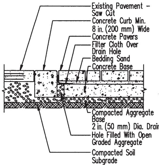
Figure 13. Crosswalk with concrete base.
