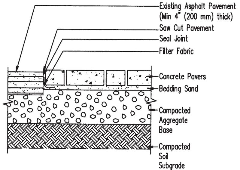
Figure 14. Crosswalk in existing asphalt pavement.
