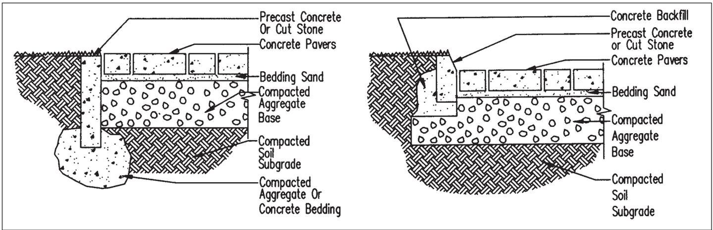
Figure 4. Precast concrete/cut stone.
