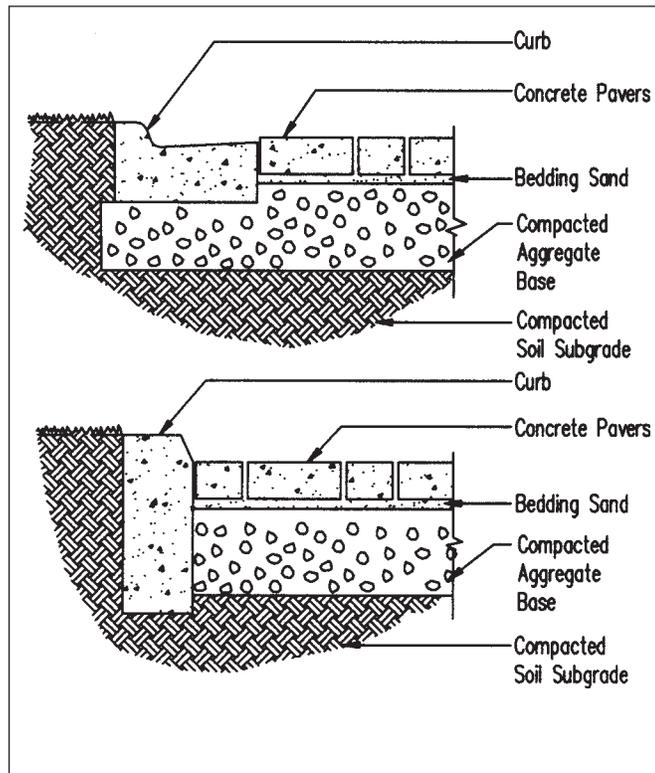
Figure 8. Poured-in-place concrete curbs.
