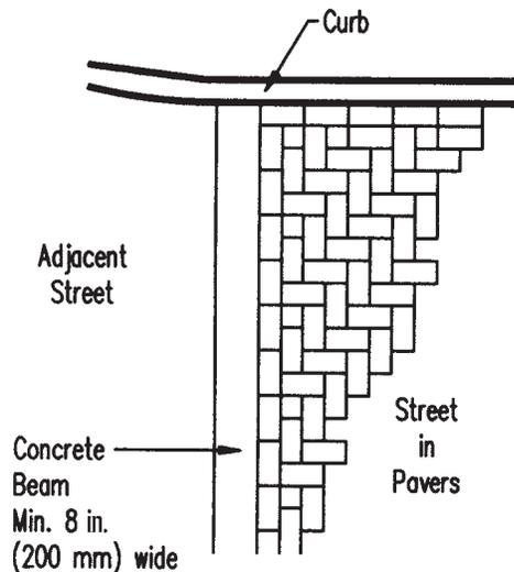
Figure 12. Concrete beam.
