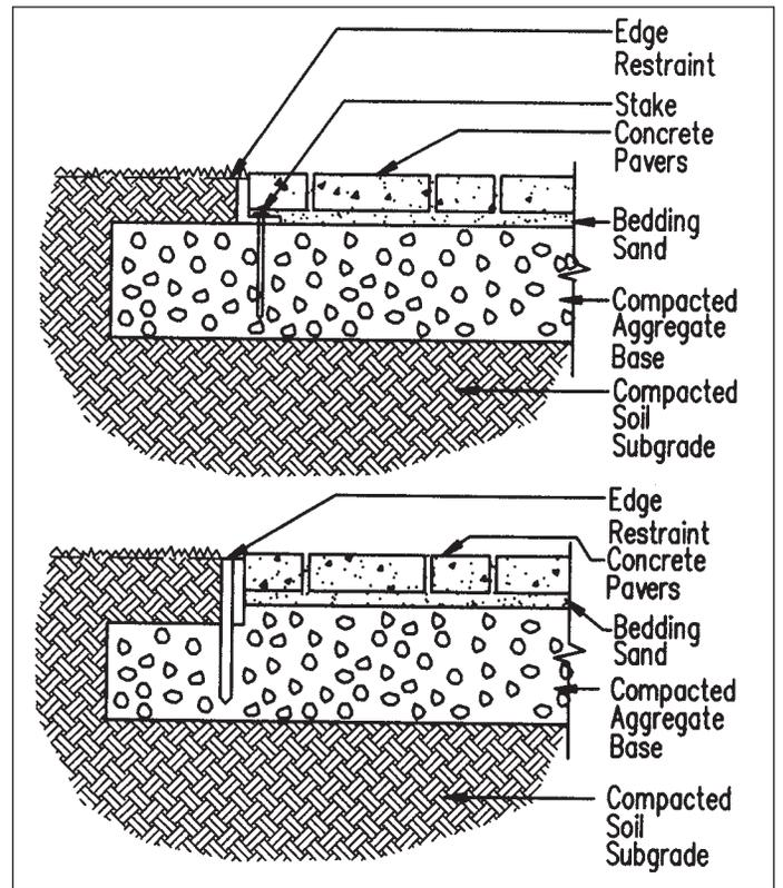
Figure 6. Aluminum and steel edging.
