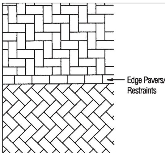
Figure 1. Change in laying pattern direction.
